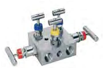
Sync-Lok 5 Valve Manifold Pipe to Pipe design for connecting system impulse lines and transmitters. This valve consists of 1/2" NPT Female connectors on 2 1/8" centers (54mm) to suit the inlet connection. This valve provides two instrument isolation valves, two equalizer valves and one bleed valve (for testing).
