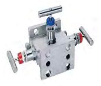
**Sync-Lok** 3 Valve Manifold Flange to Flange design for connecting system impulse lines and transmitters, This valve consist of Flange to Flange connections on 2 1/8" (54mm) centers and one equalizer valve and two block valves.
