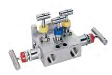
Flange design for connecting system impulse lines and transmitters. This valve consists of Pipe to Flange connections with Teflon/Viton O-Ring packing on 2 1/8" centers (54mm) to suit the inlet connection. This valve provides two instrument isolation valves, two equalizer valves and one bleed valve (for testing).
