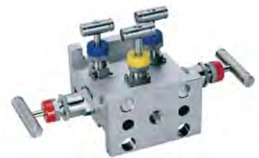
Sync-Lok 5 Valve Manifold Flange to Flange design for connecting system impulse lines and transmitters. This valve consists of two Flange connections with Teflon/Viton O-Ring packing on 2 1/8" centers (54mm) to suit the inlet connection. This valve provides two instrument isolation valves, two equalizer valves and one bleed valve (for testing).
