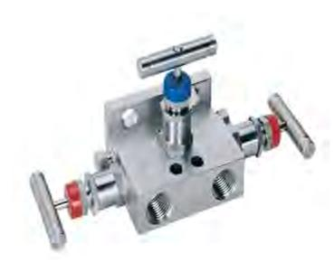
**Sync-Lok** 3 Valve Manifold Pipe to Flange design for direct mounting, connecting system impulse lines and transmitters, This valve consist of 1/2" NPT Female connections on 2 1/8" (54mm) centers and one equalizer valve and two block valves. 1/4" NPT purge connections (2) optional.
