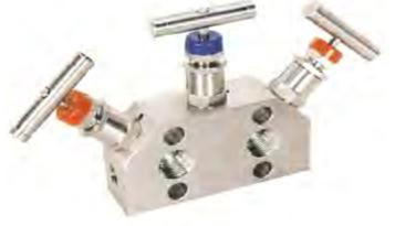
**Sync-Lok** 3 Valve Manifold Pipe to Flange, base mount connection design for connecting system impulse lines and transmitters, This valve consist of 1/2" NPT Female connections on 2 1/8" (54mm) centers and one equalizer valve and two block valves.
