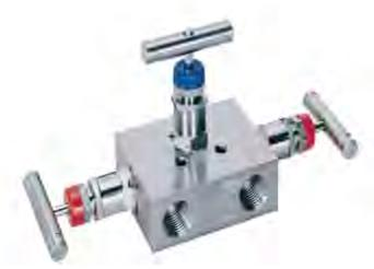
**Sync-Lok** 3 Valve Manifold Pipe to Pipe design for remote mounting, connecting system impulse lines and transmitters, This valve consist of 1/2" NPT Female connections on 2 1/8" (54mm) centers and one equalizer valve and two block valve.
